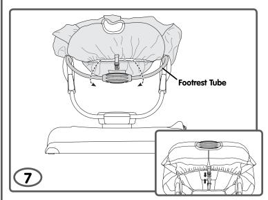
• Fit the lower pocket on the pad around the footrest tube. Fasten the straps underneath the footrest tube to secure the lower portion of the pad.
